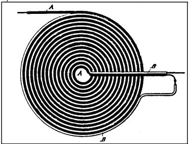
5. Coil for Electro-Magnets
